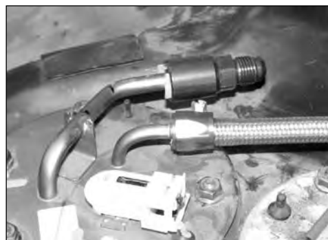
Figure 16 - Connect Return Hose to Fuel Pump
