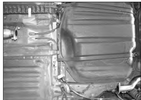
Figure 6 - Exhaust Midpipe Removal
