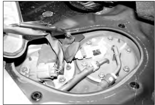
Figure 5 - Fuel Pump Access Cover Removed
