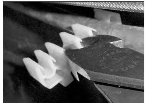
Figure 14 - Cutting Fuel Line Support Clips
