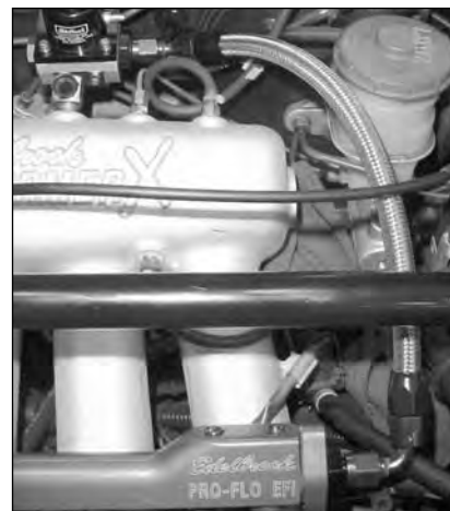
Figure 19 - Fuel Rail to Regulator Line
