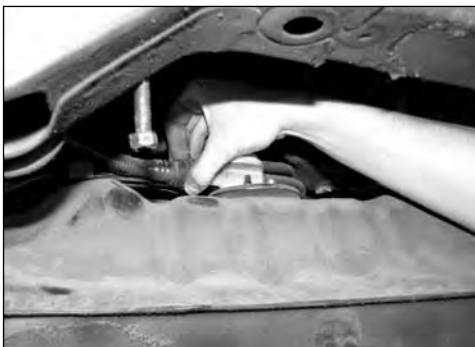
Figure 8 - Tank Vent Hose Removal
