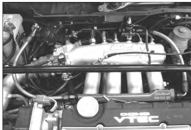
Figure 8 - Overall Fuel Line Routing
