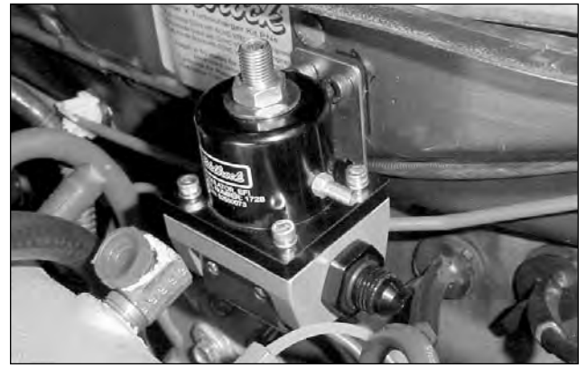
Figure 4 - Regulator Mounted on Firewall
