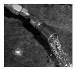
7. Install on vehicle and turn key on to pressurize fuel system (Do not start engine). Check for leaks.
