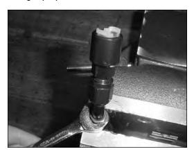
2. Remove socket from vise and then remove socket from hose by pulling and twisting clockwise.
