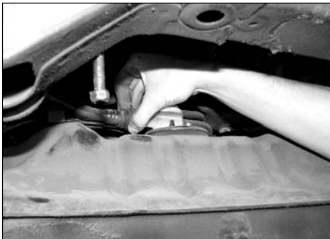
Figure 8 - Tank Vent Hose Removal
